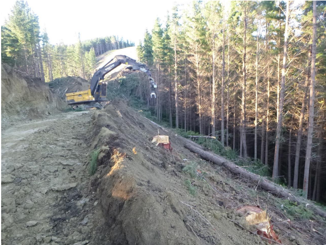
Photo 9: Log 19 shovelling stems into reach for the skidder for extraction to Landing 18.
