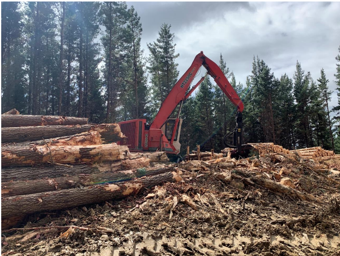
Photo 10: Log 16 Madill processor working on Landing 33.
