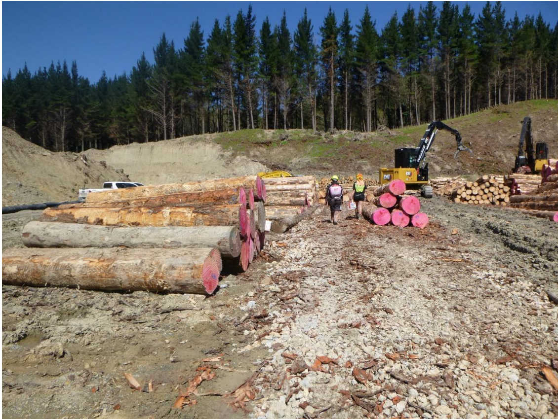
Photo 3: Log 19 operating on Landing 10 with Tui spraying antisapstain and Brooke stencilling butts of logs.
