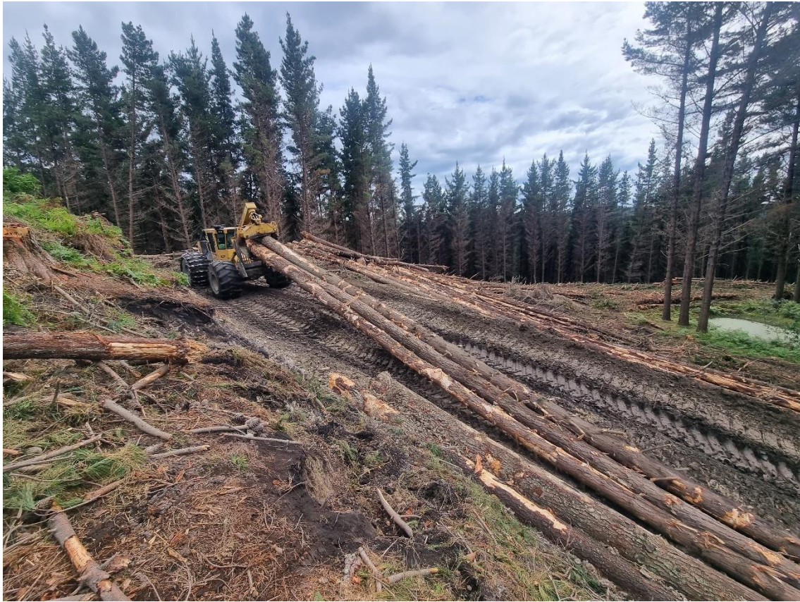
Photo 3: Skidder extracting a good size drag back to the landing for processing at Landing 31.
