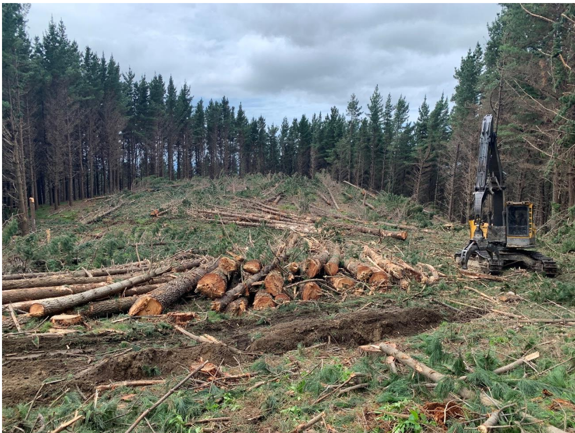
Photo 4: Log 16 Volvo bunching logs for the Tigercat skidder.
