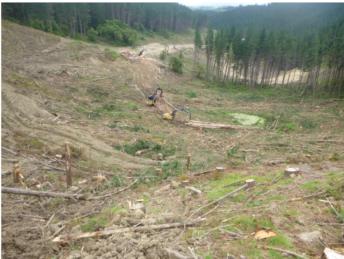
Photo 8: A & R Logging crew, Log 19 extracting stems from Setting 500 back to Landing 9 with shovel machine and falling machine.
