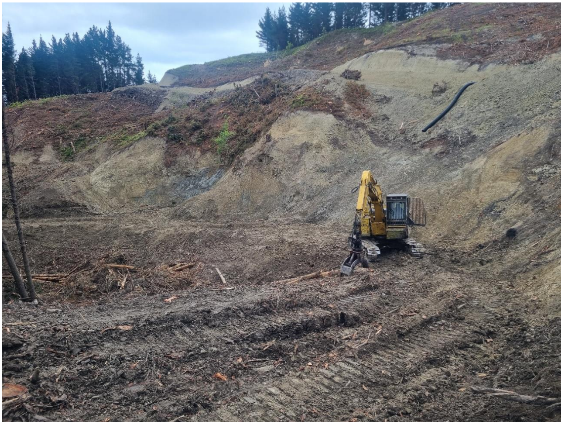
Photo 4: Shovel machine down on extraction track pulling stems from roadlining operation.
