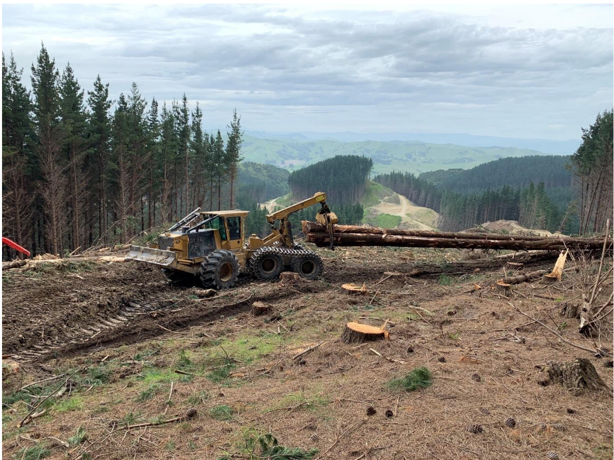
Photo 8: Log 16 Tigercat skidder pulling drag back to Temporary Landing 2.
