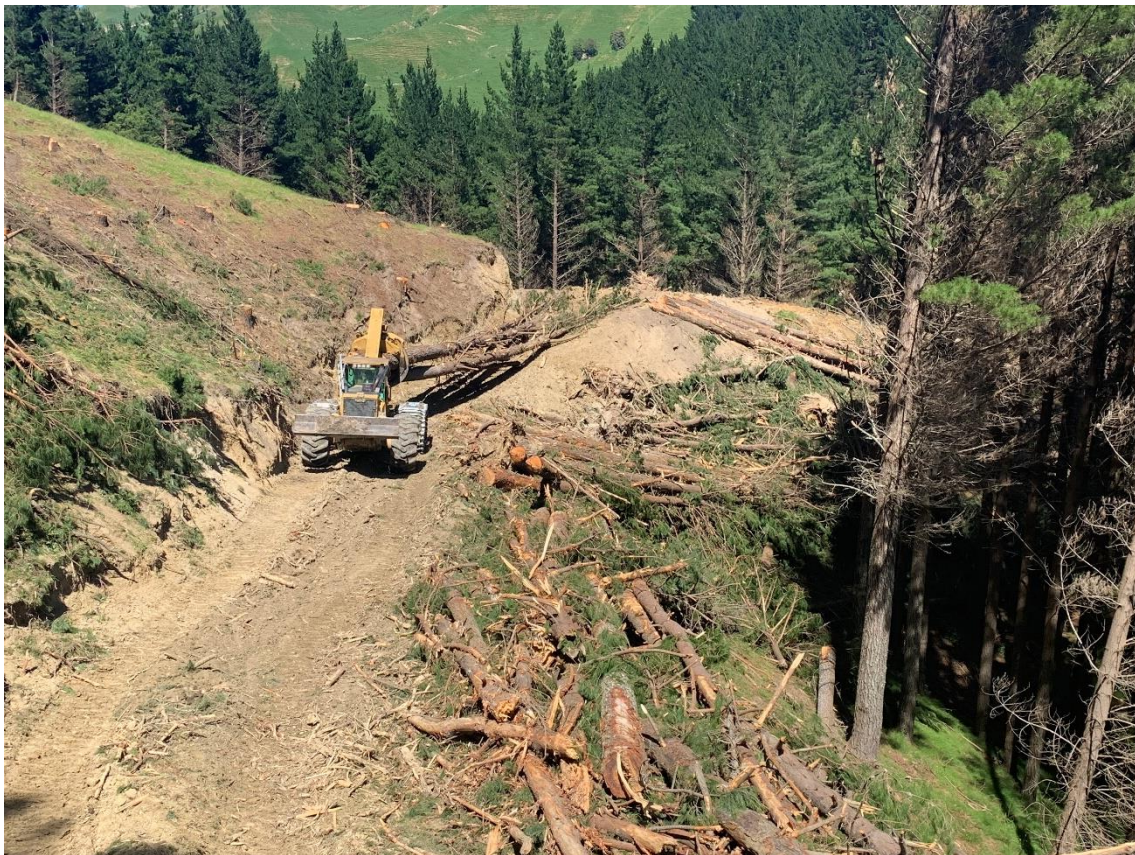
Photo 6: Log 16 Tigercat skidder extracting logs from Setting 518.
