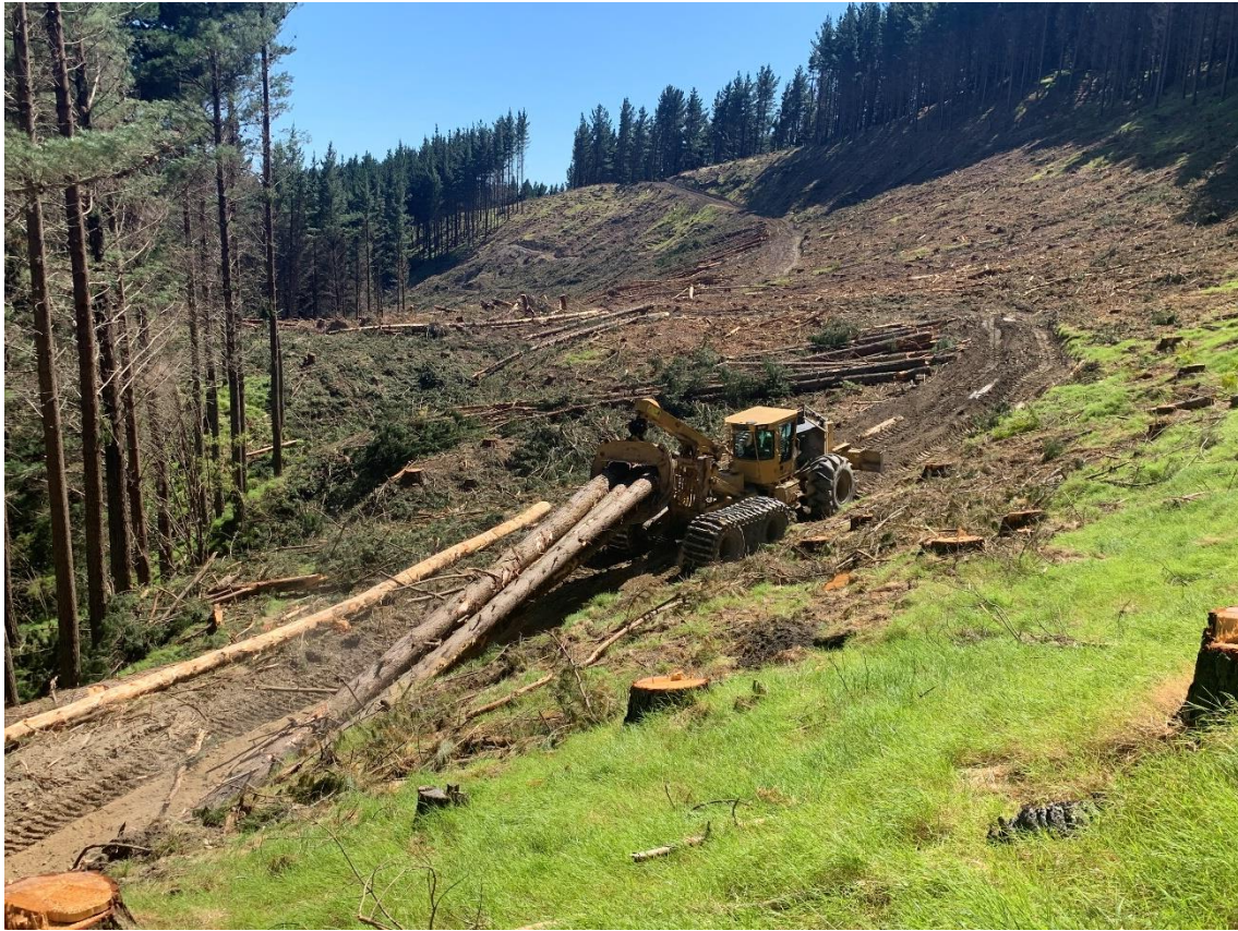
Photo 7: Log 16 Tigercat skidder extracting logs from Setting 518.
