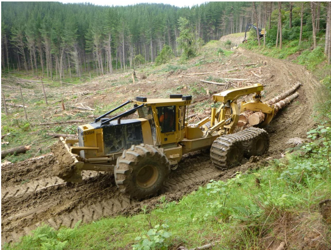
Photo 4: Log 19 extracting stems from Setting 500 back to Landing 8.
