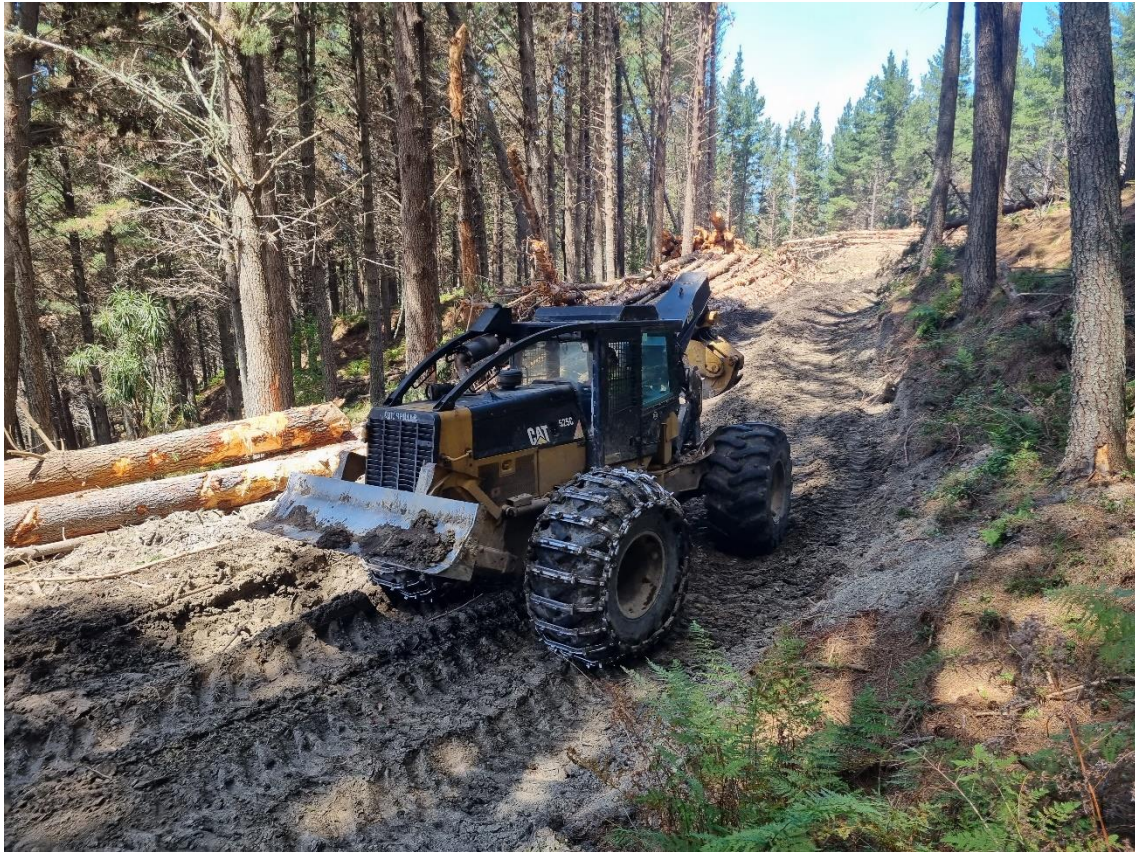
Photo 3: Skidder extracting stems to Landing 21.
