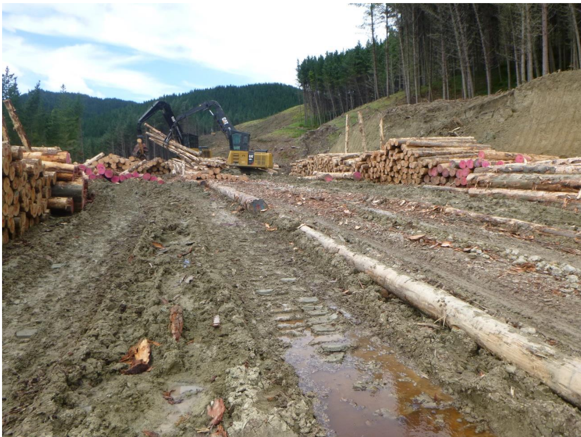
Photo 6: A & R Logging crew, Log 19 processing and fleeting stems on Landing 7.
