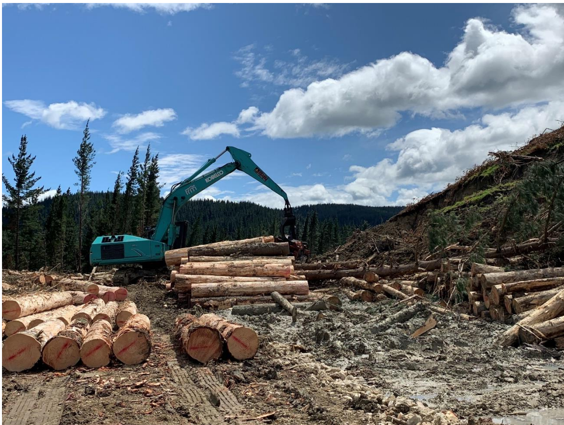
Photo 8: Processor with Woodsman head at work.
