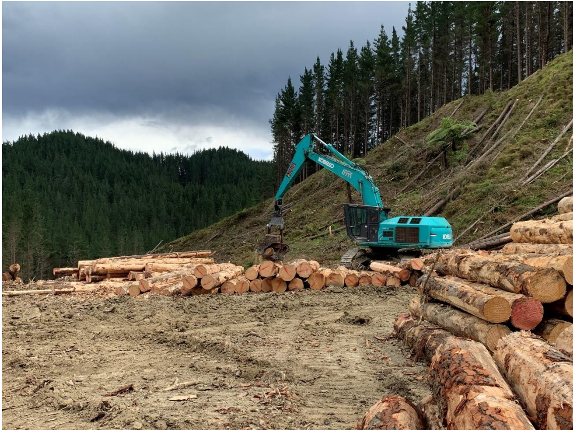
Photo 11: Kobelco with Woodsman head working on Temporary Landing 1.
