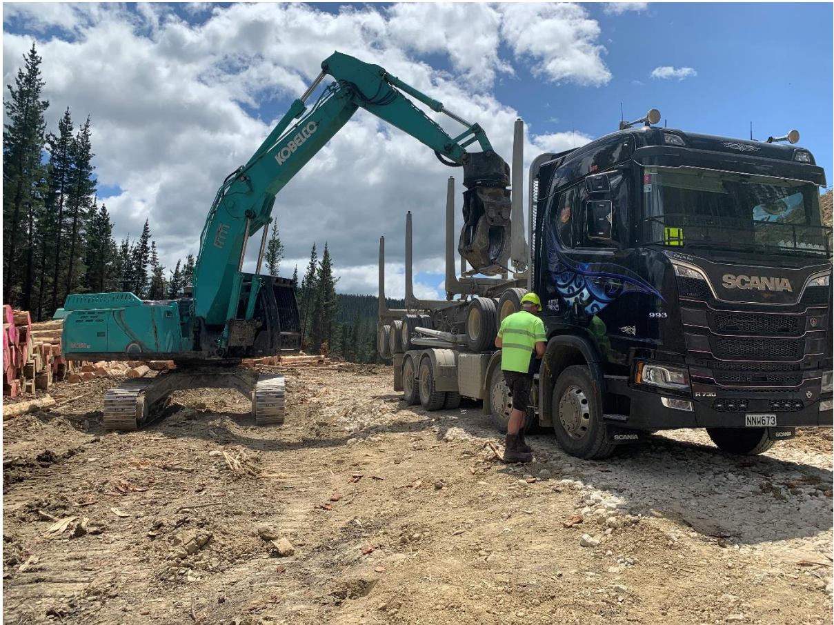
Photo 2: Log 6 loader pulling trailer off log truck on Landing 10.
