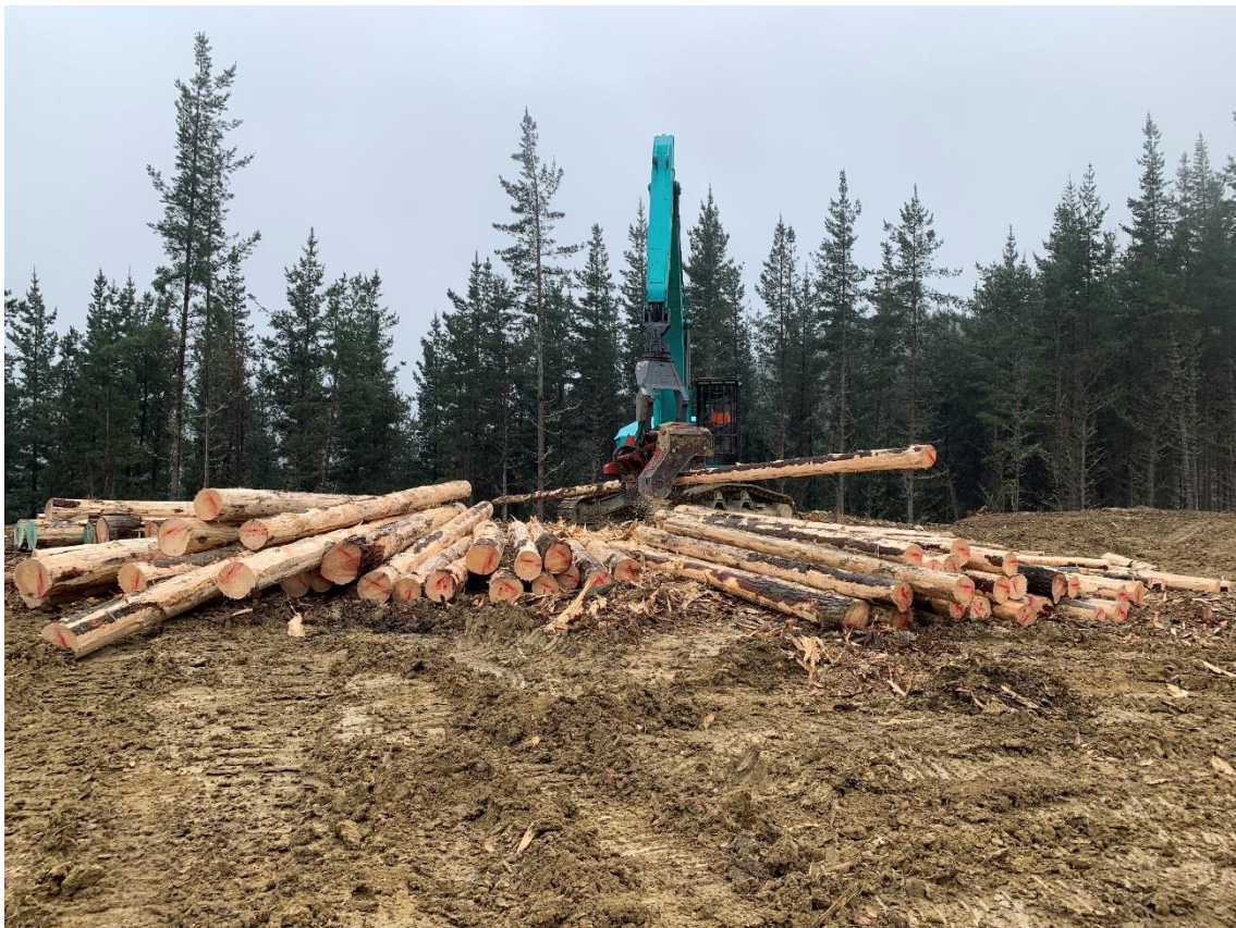
Photo 6: Kobelco processor with Woodsman head working on Landing 5.
