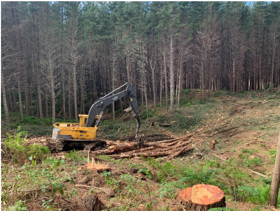
Photo 6: Log 16 300 Volvo bunching logs for skidder in Setting 507.
