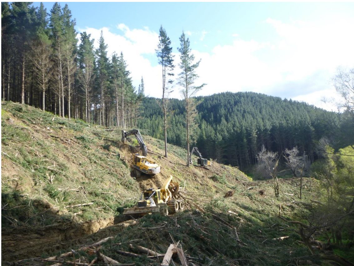
Photo 4: Log 19 in Setting 500, using the shovel machine to “heal” in a track so the falling machine can access and fall the last two stems, and pass these down to the skidder for extraction to Landing 105.
