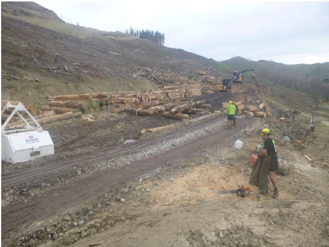
Photo 2: Log 19 operating on Landing 1 – manually processing oversized edge trees and loading out logs.
