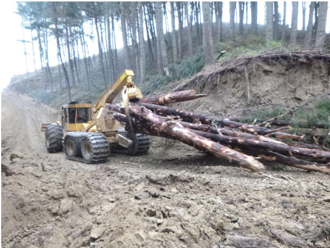
Photo 4: A & R Logging crew, Log 19 extracting stems with a 6-wheeled skidder from Setting 500 to Landing 2.
