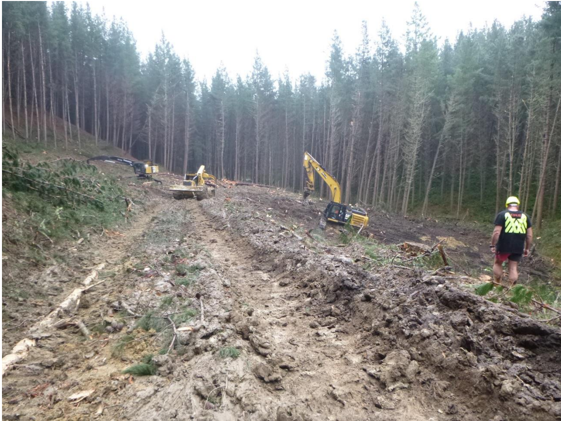
Photo 3: A & R Logging crew, Log 19 operating in roadline Setting 500 – falling and shovelling stems to the skidder for extraction.
