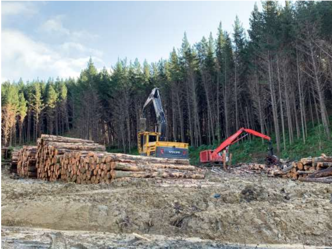
Photo 5: Volvo 250 and Madill processor working on Landing 6, Clarke Road.
