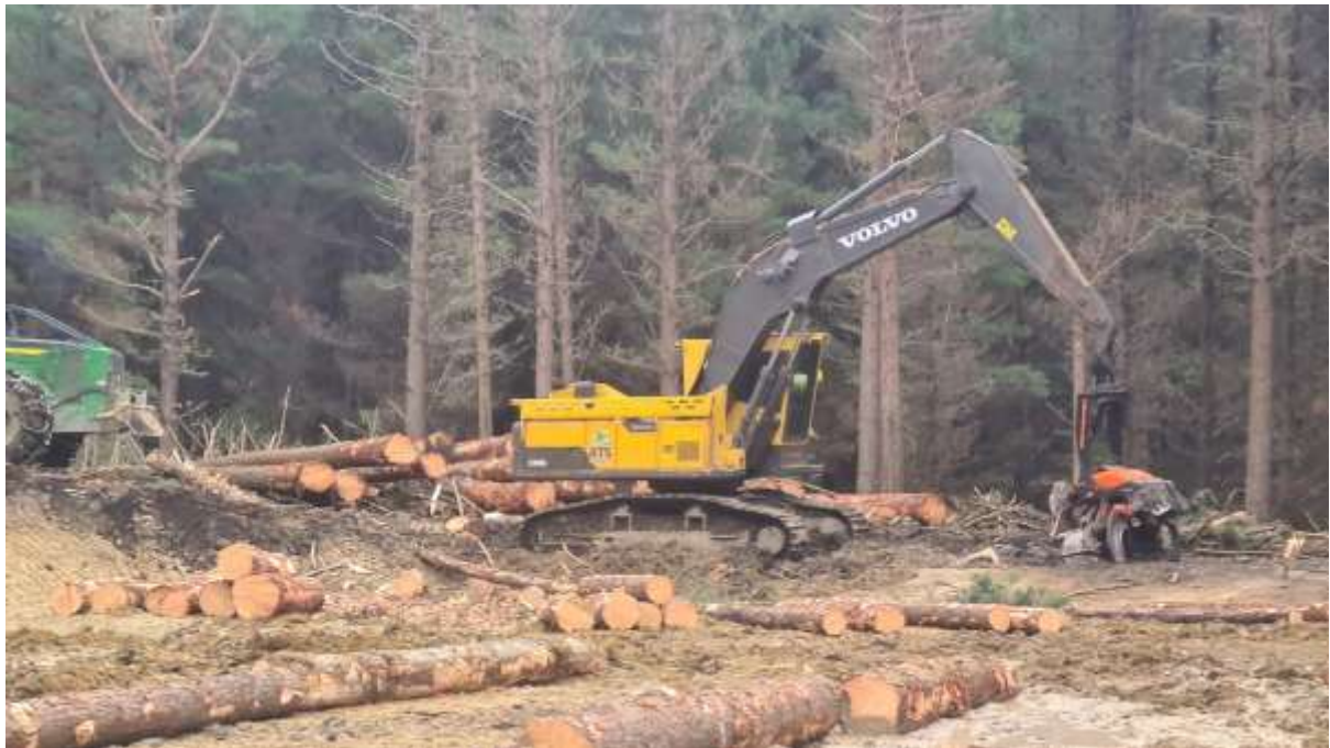
Photo 3: Processor on Landing 61.
