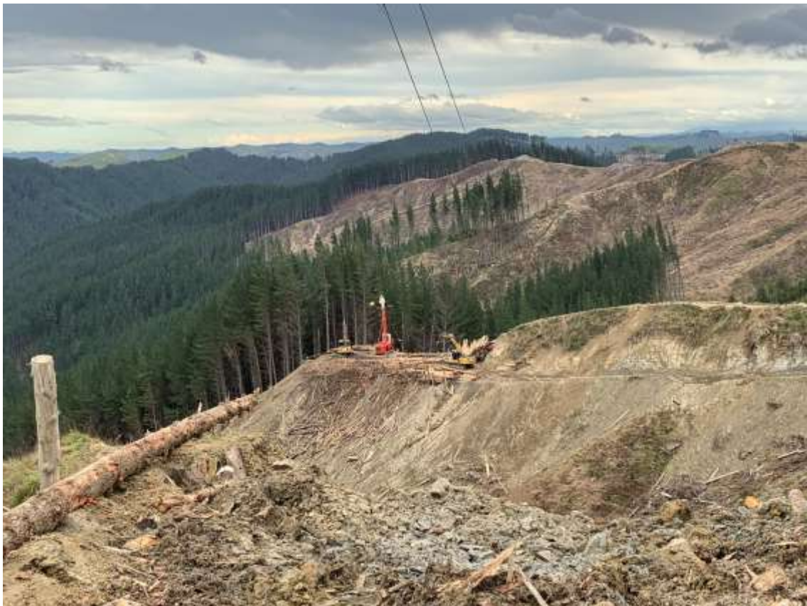
Photo 6: Madill 171 with CAT processor and loader on Landing 605.
