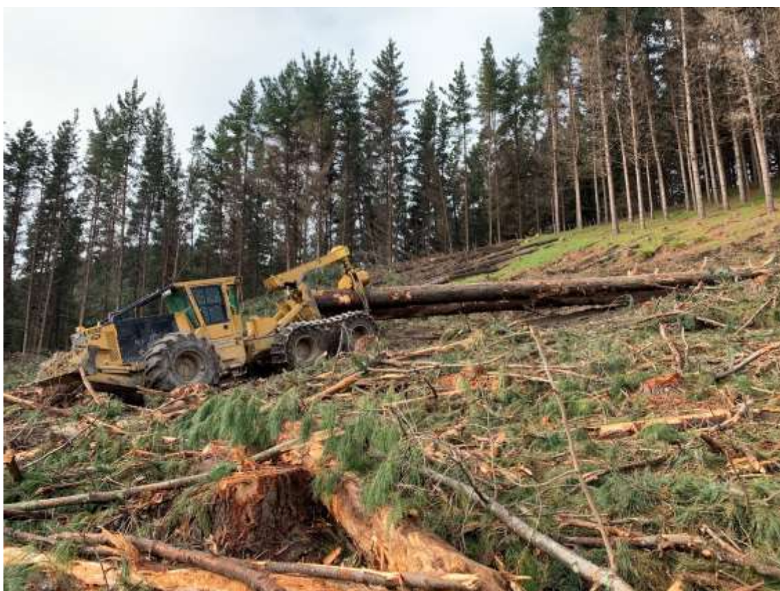
Photo 2: Log 16 Tigercat 625E hauling drag to Landing 1.
