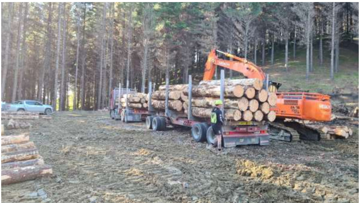
Photo 2: Truck driver chaining load on Landing 61.
