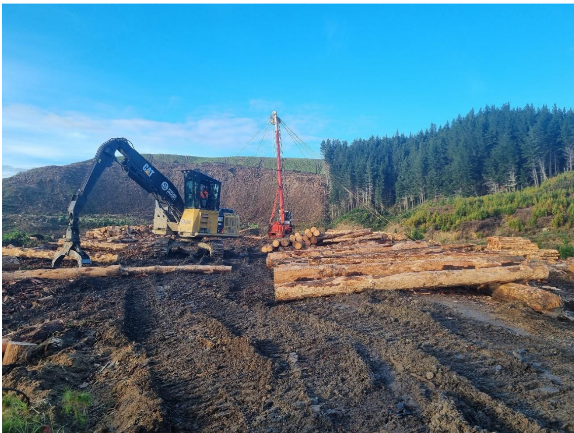
Photo 2: Excavator laying logs out to be quality checked and graded on Landing 120.
