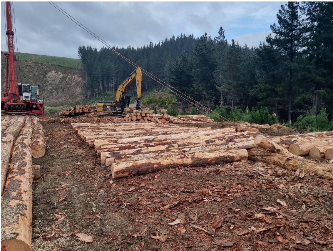
Photo 2: Madill 172 Tower hauler on left and excavator fleeting logs on landing.
