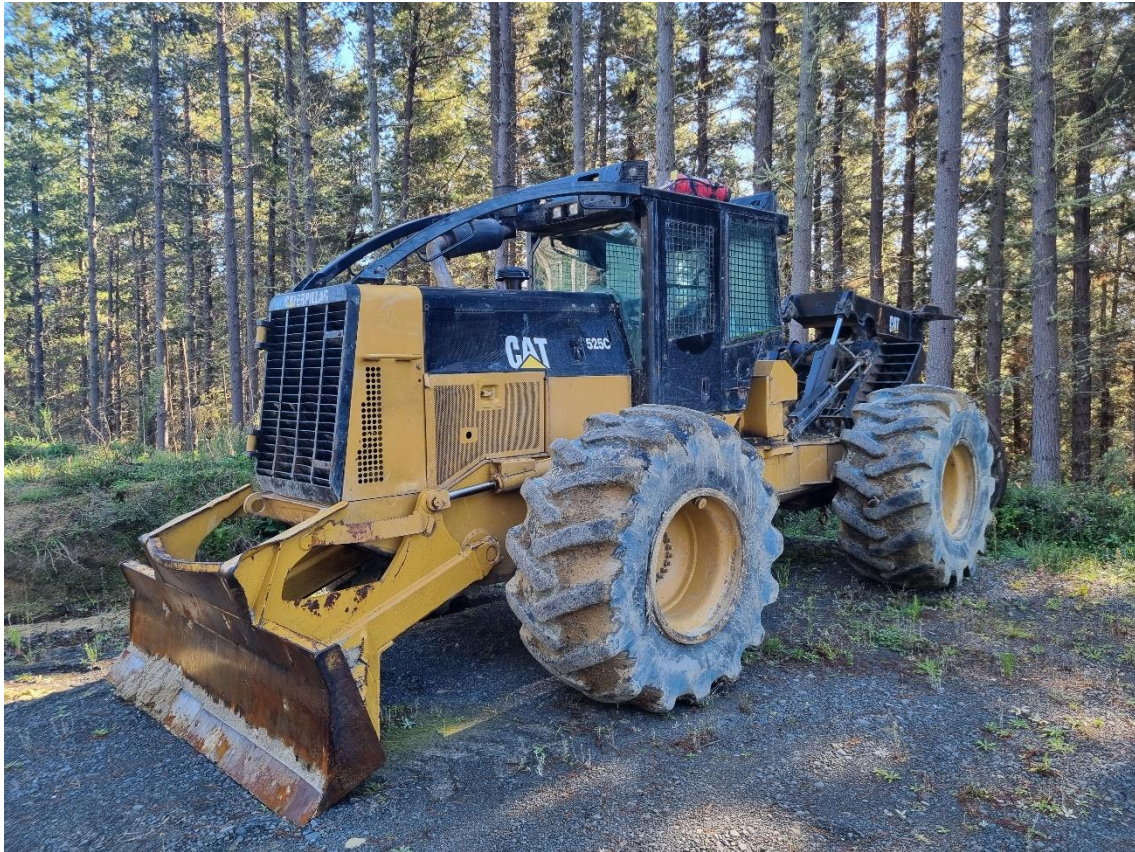
Photo 3: Cat 525C skidder used to two-stage wood over a longer distance than a loader would shovel.
