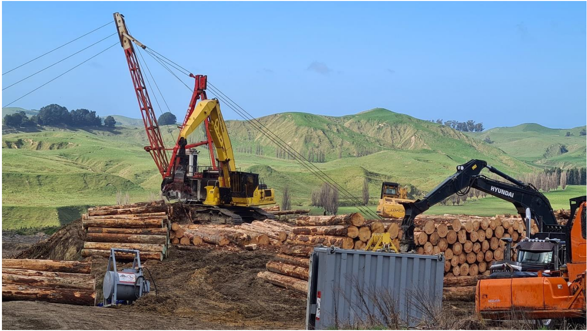
Photo 3: Swing yarder, grapple loader and processor at work on Landing 18.
