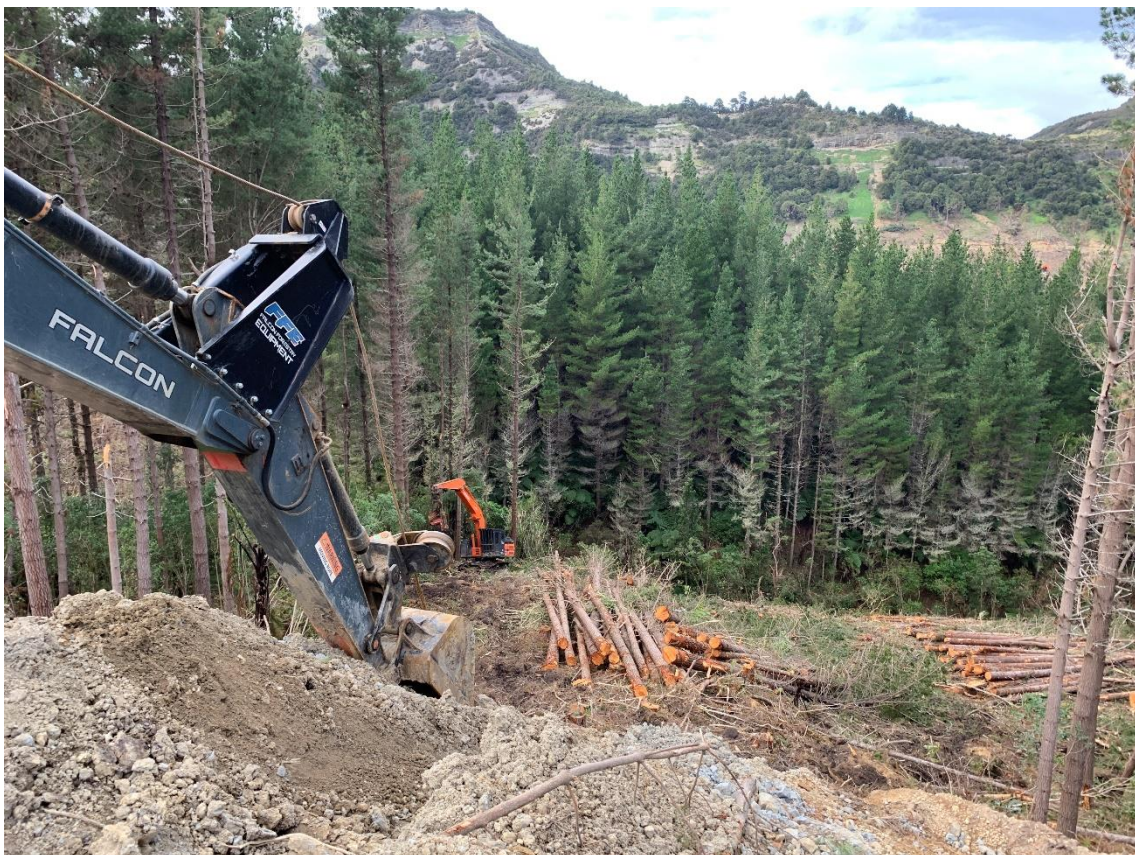
Photo 2: Setting 68 being opened up and bunched by felling machine.
