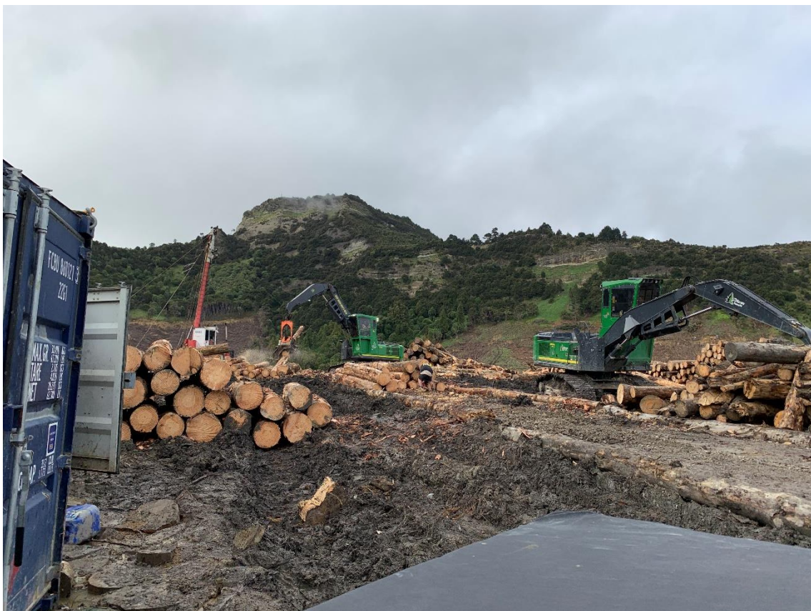
Photo 6: Processor cutting logs on Landing 69.
