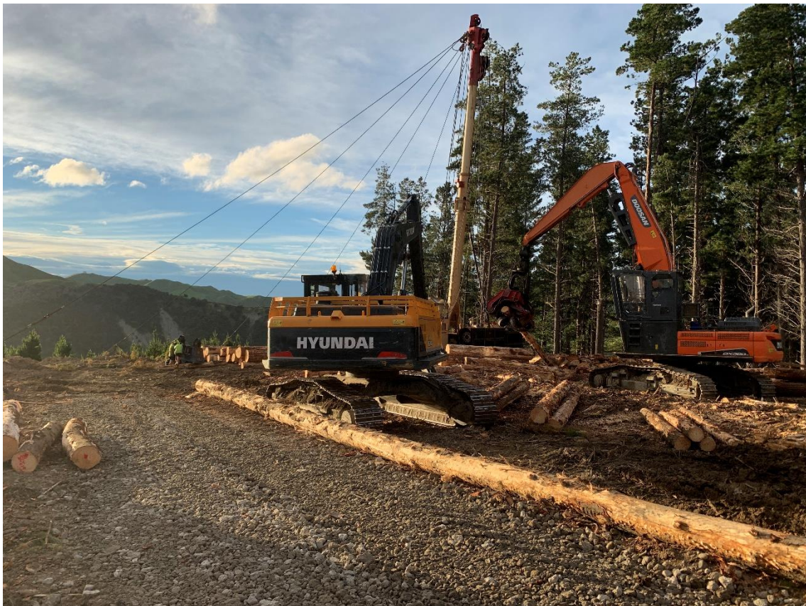
Photo 4: Hauler guy ropes run, carriage maintenance before they attach to sky.
