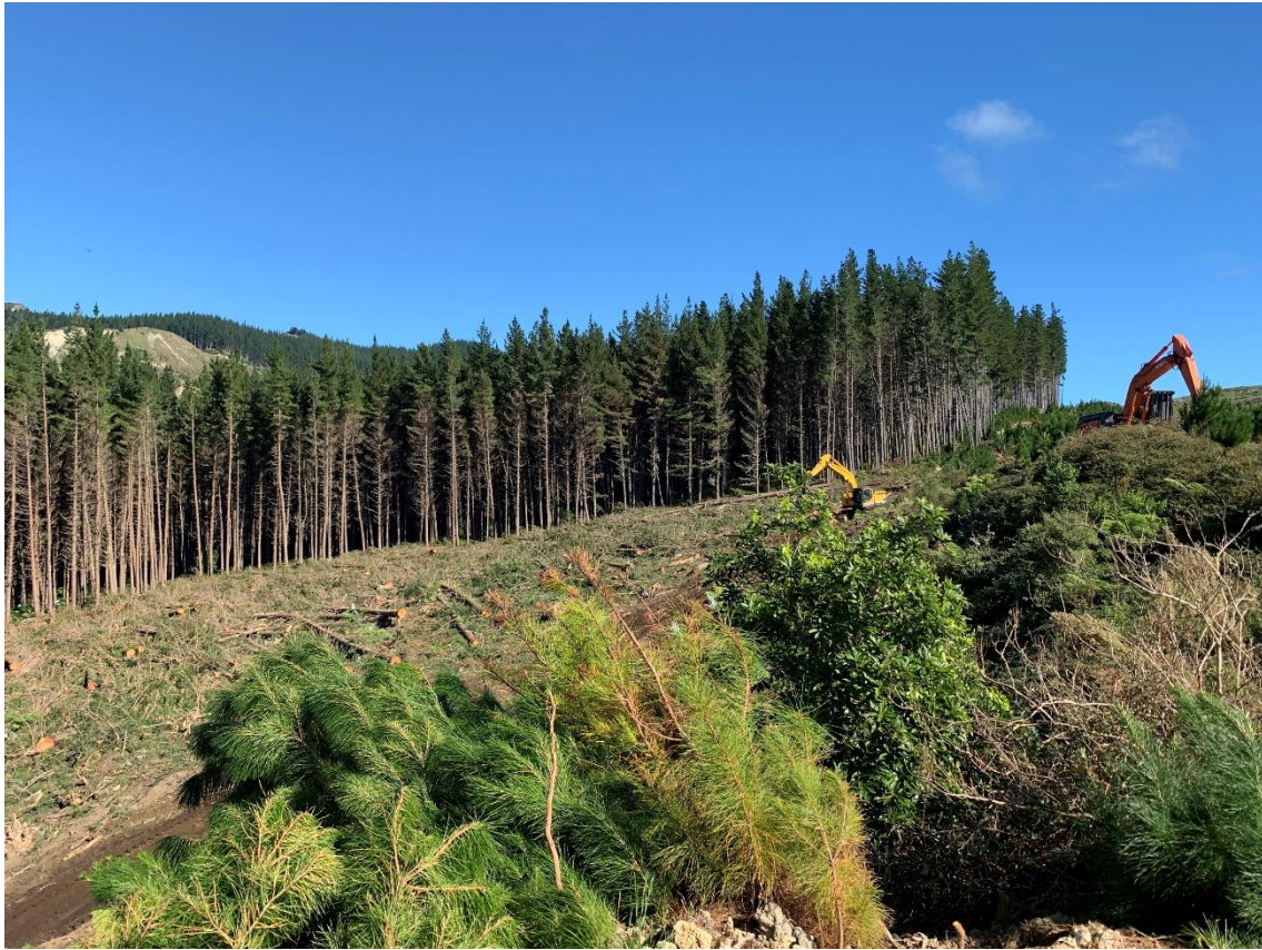
Photo 3: Shovel machine in Setting 17, shovelling wood while hauler is set up.
