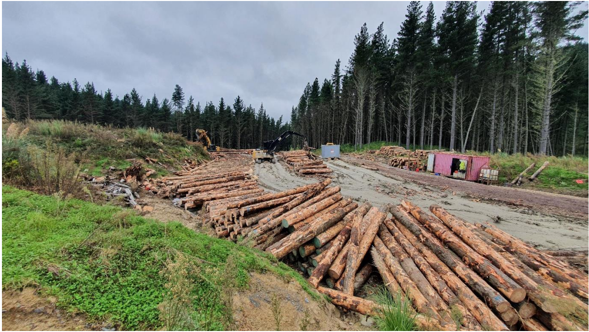
Photo 1: Log 1 working in wet conditions shovelling logs, fleeting and stacking on Landing 9.
