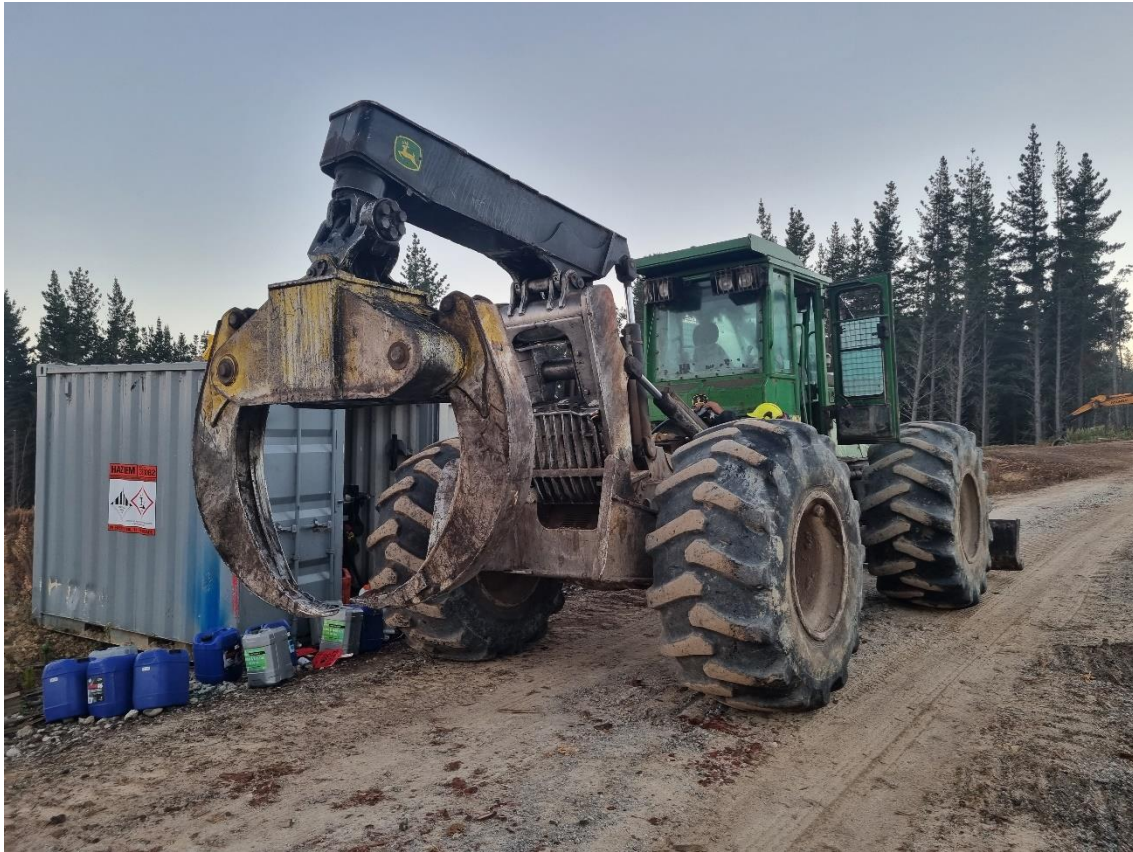
Photo 1: Skidder machine used to two-stage wood from one location to another to facilitate loadout.
