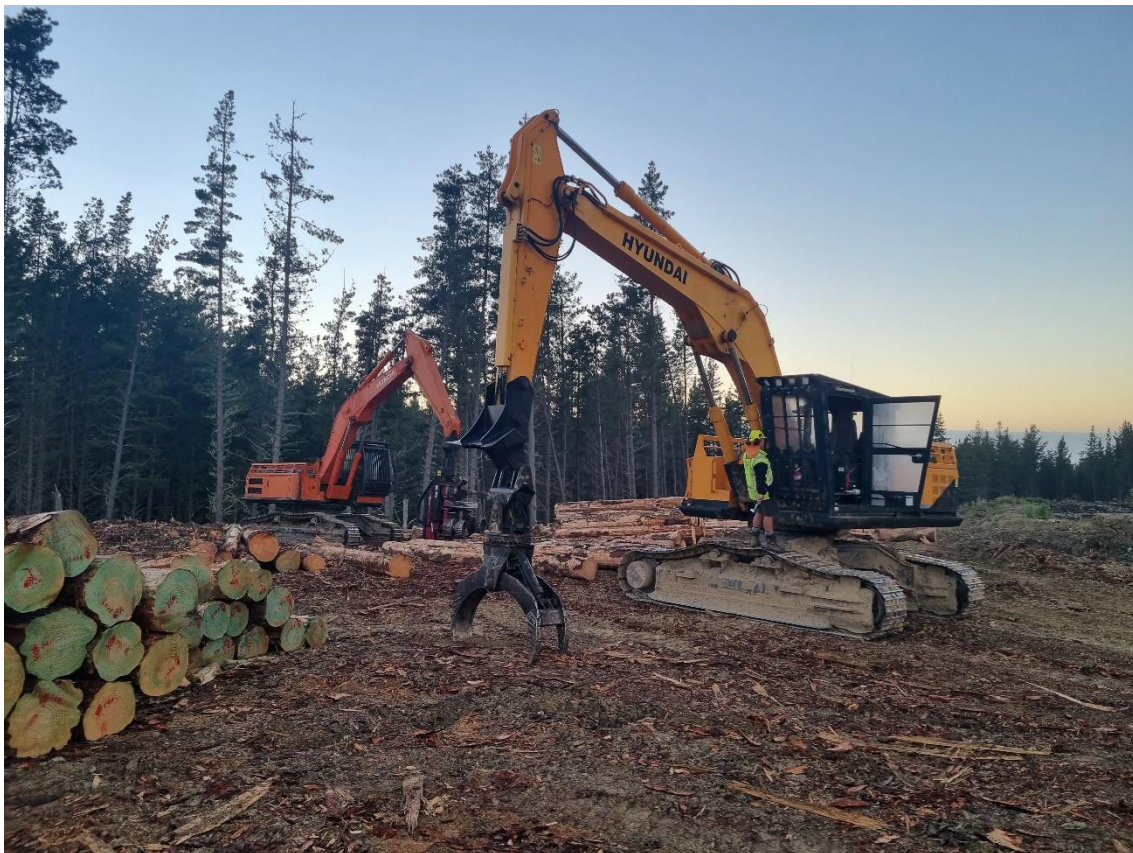
Photo 2: Processor and loader machines on Landing 56.
