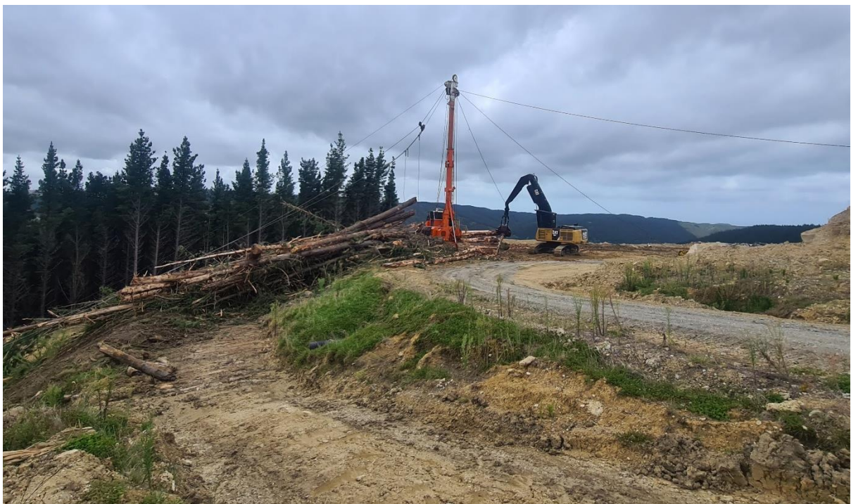
Photo 2: Swing yarder at work on Setting 8.
