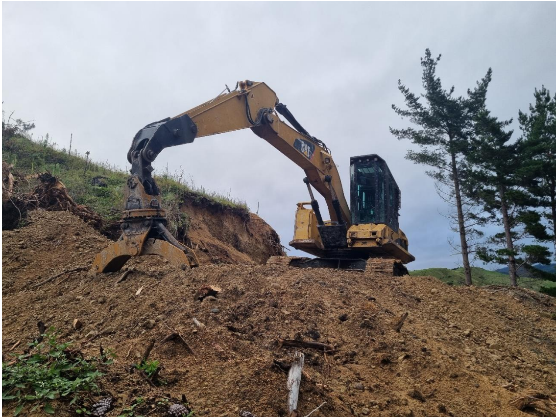
Photo 5: Excavator with a grapple head used to shovel wood from harvestline chute to landing.
