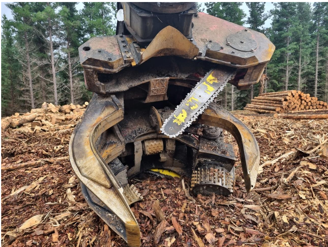
Photo 6: Inside look at the processor head.
