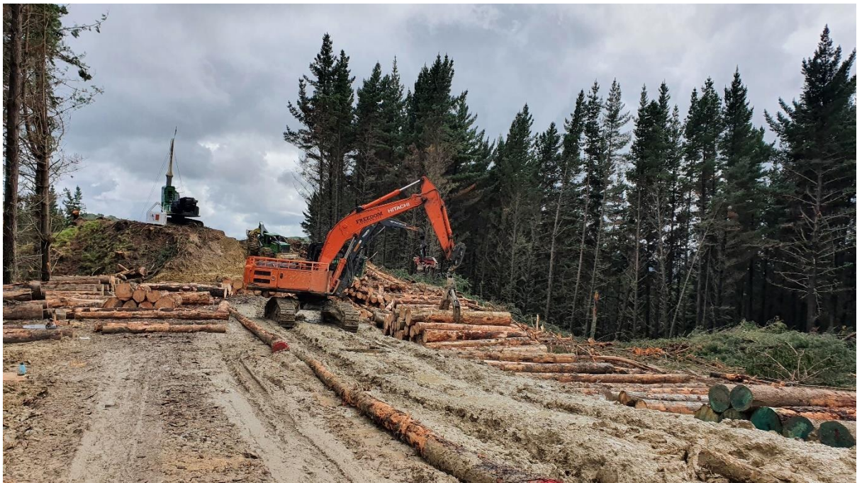
Photo 8: Fleeting and stacking logs on Landing 17.
