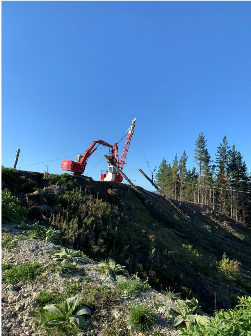
Photo 5: A & R Logging crew, Log 27 swing yarder hauling up drag and excavator moving them to be processed.
