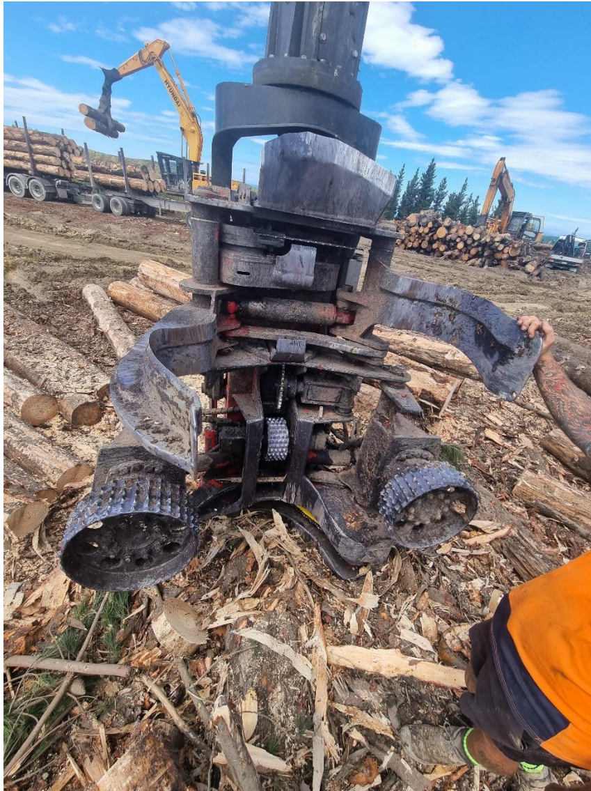
Photo 3: A rare look into the processor head while calibration is carried out.
