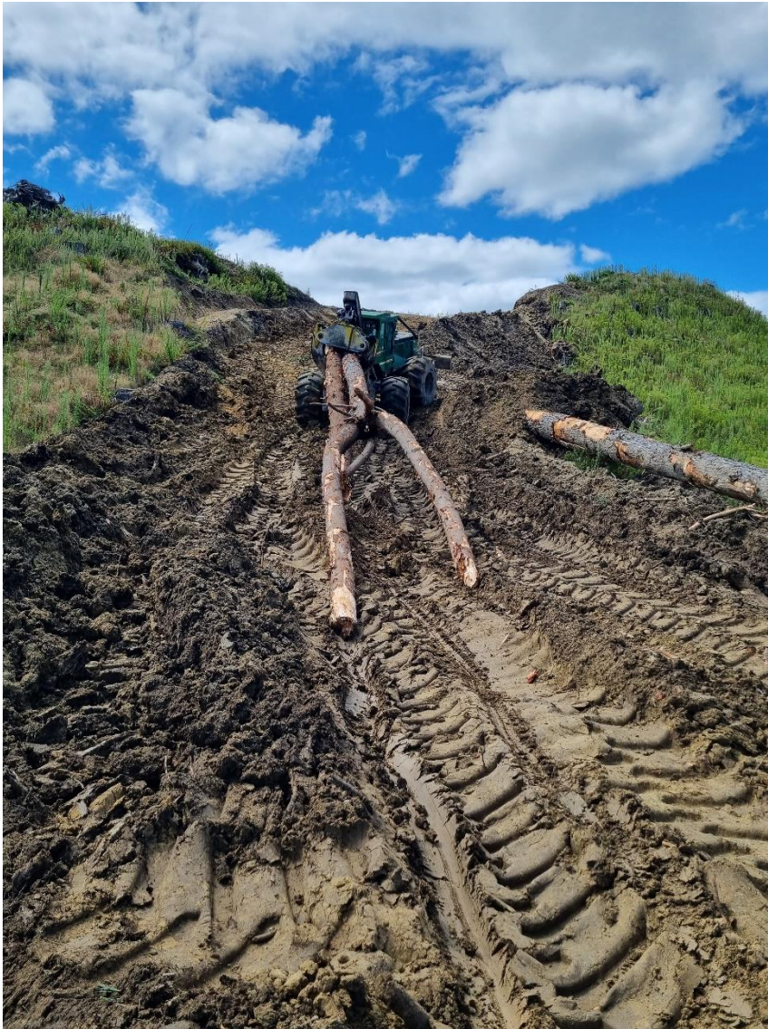
Photo 8: Grapple skidder making its way out of a two-stage climb taking stems from Pad 56A to Landing 56.
