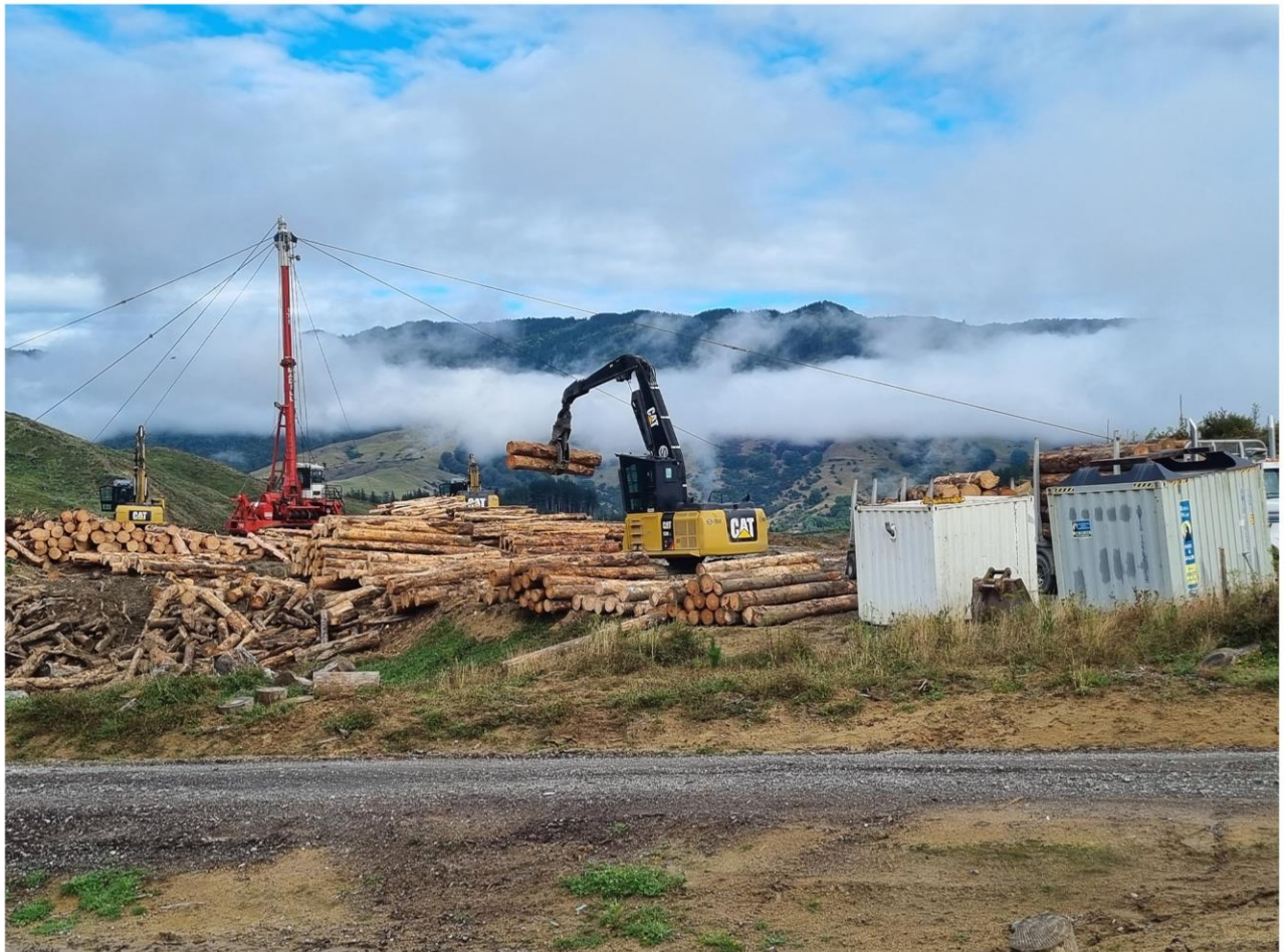
Loader carrying and sorting out logs on Landing 80.
