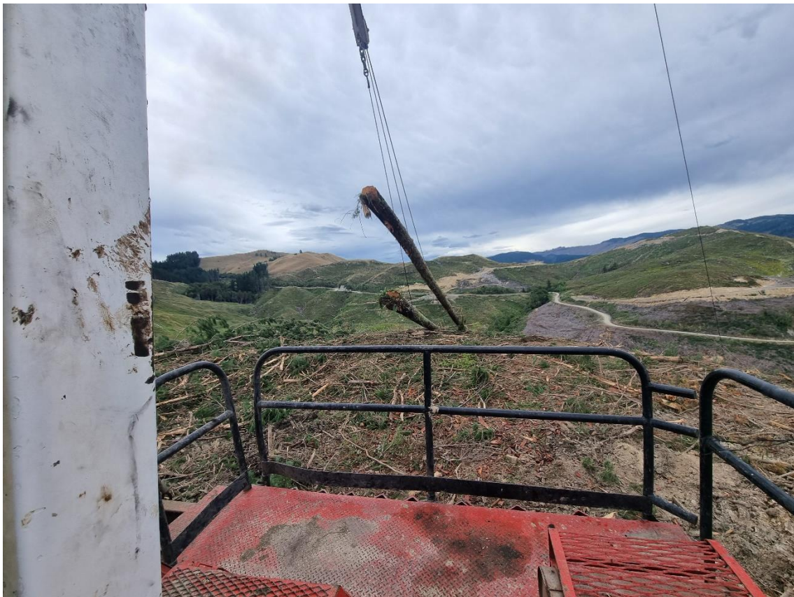
Photo 2: Stems on the in-haul about to be landed.
