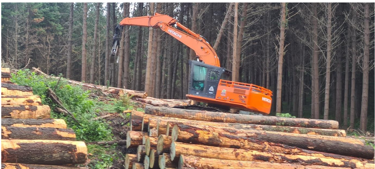
Photo 3: Roadline Setting 510, wood being shovelled to landing.
