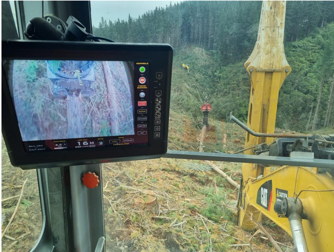
Photo 7: View from inside the harvestline machine, note the screen showing the camera view on the carriage.
