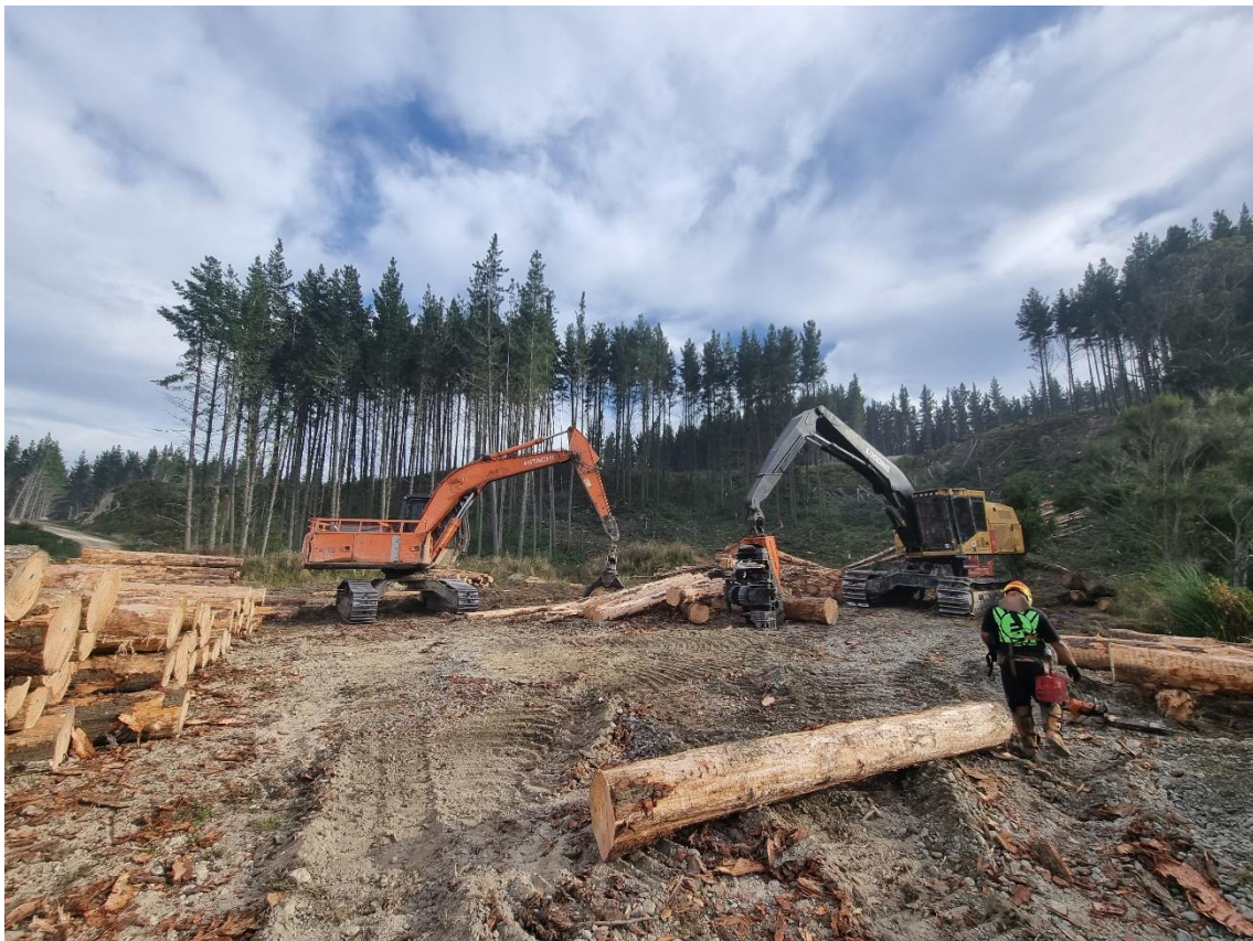
Photo 2: Processor and loader sorting log stacks on Landing 1.
