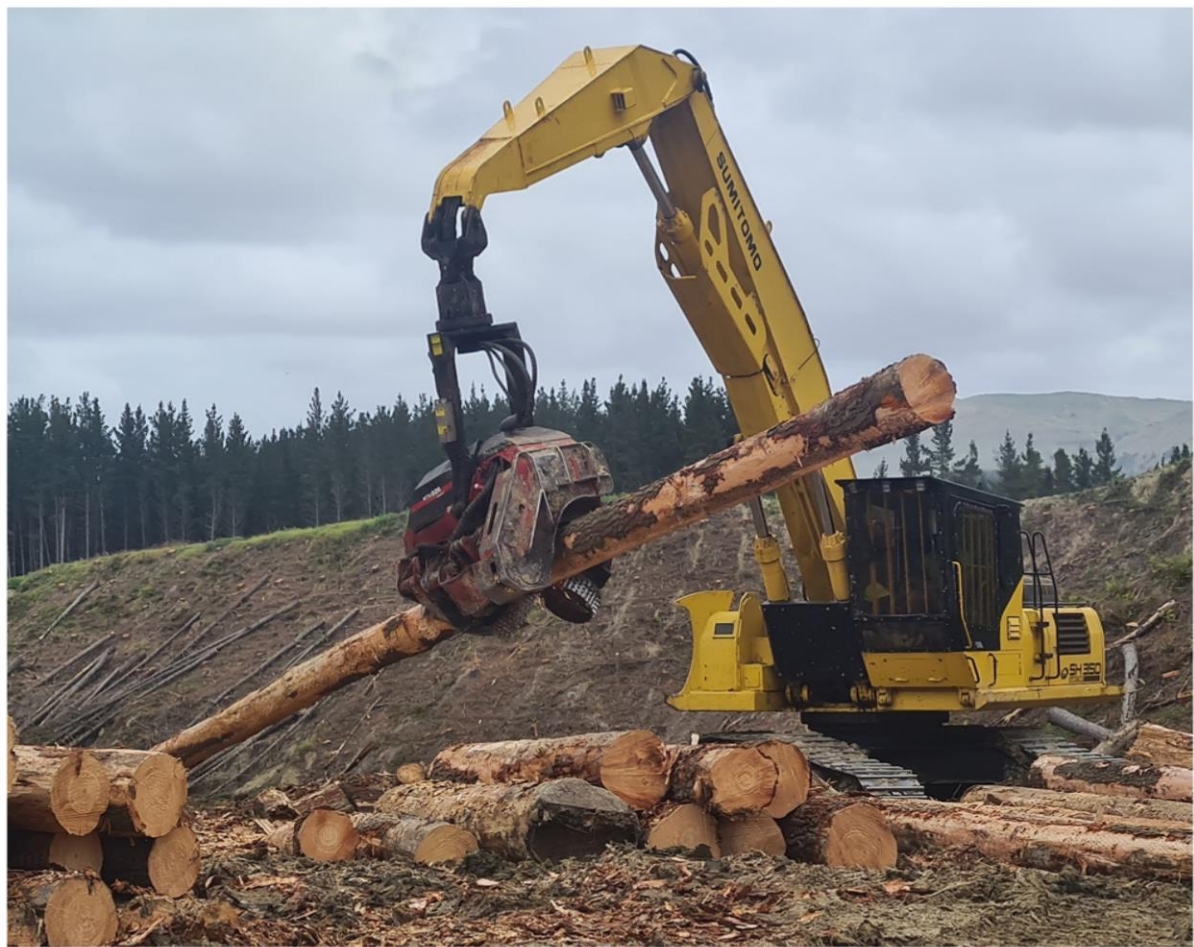
Processing logs on Landing 1.
