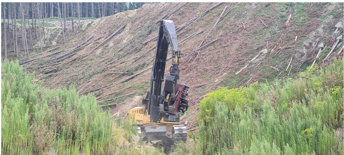
Photo 3: Felling machine coming out of Setting 21 for refuelling, felled stems in the background.
