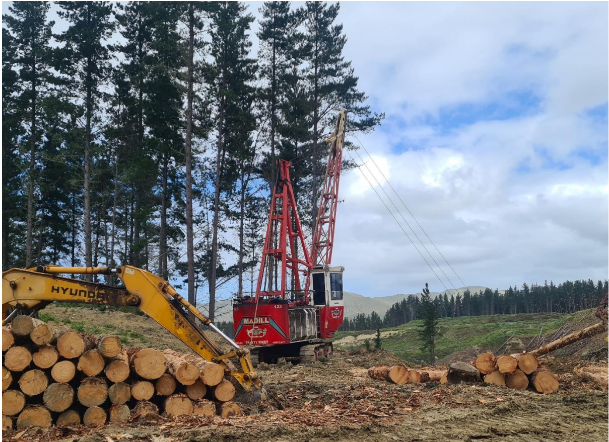
Photo 9: Swing yarder hauling in stems.
