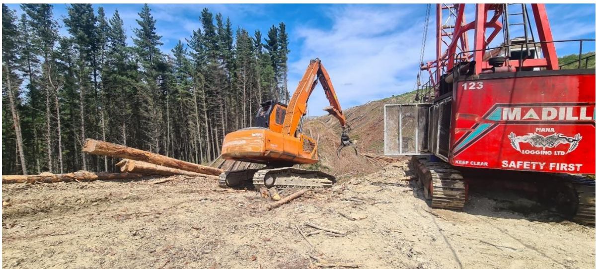
Photo 5: Excavator clearing stems from the swing yarder on Landing 21.
