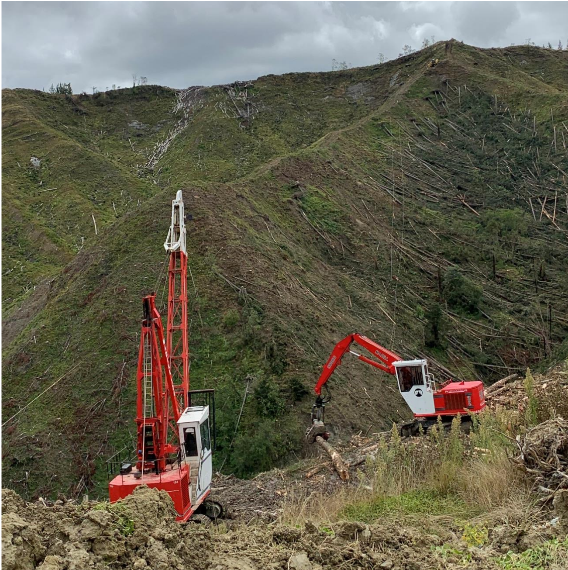
Photo 7: Swing yarder hauling in stems and processor processing stems into logs.
