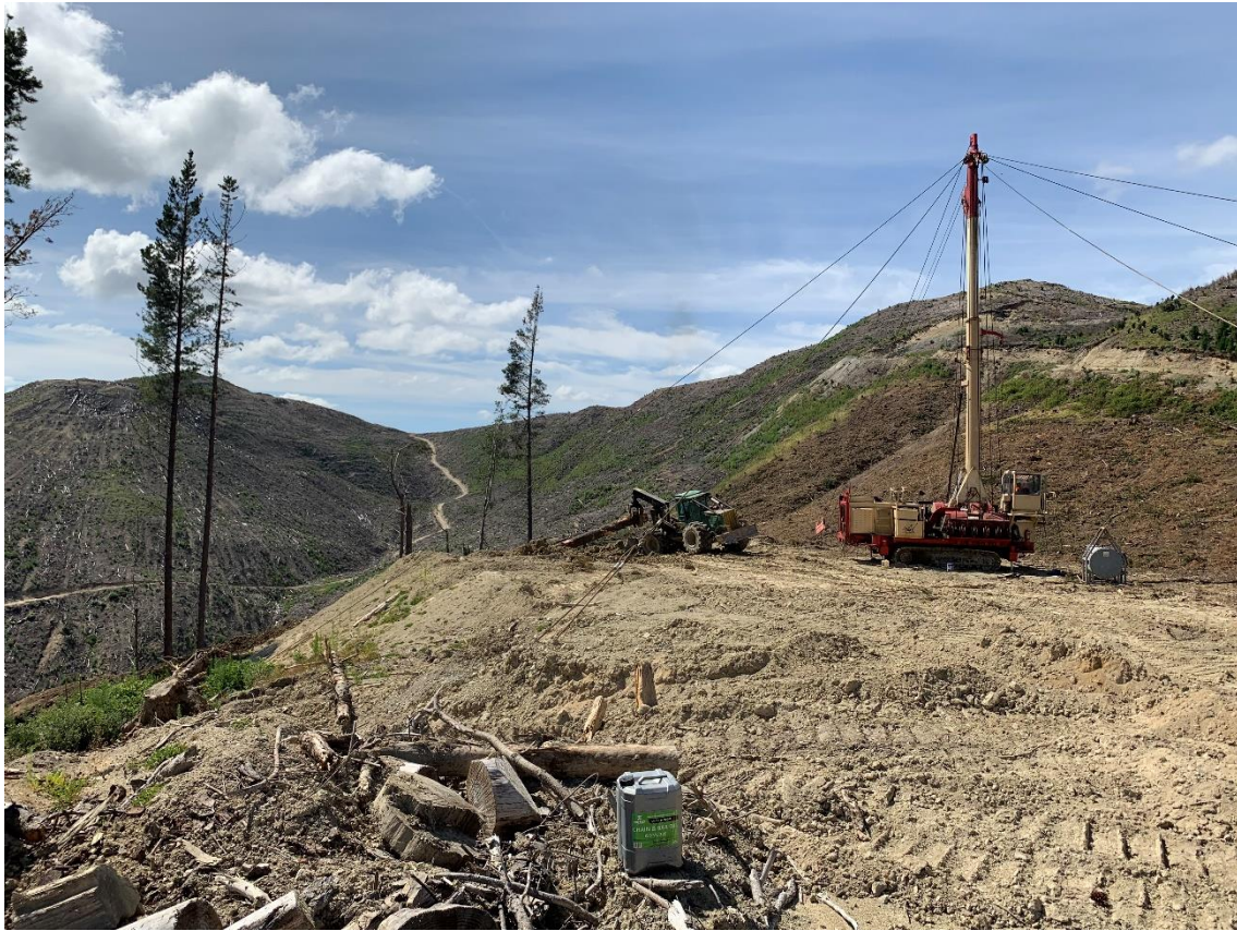
Photo 1: Skidder clearing the chute for the hauler.
