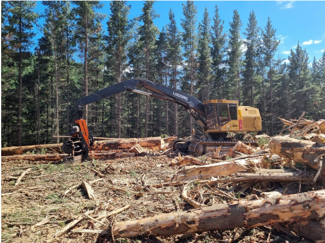
Photo 1: The multi-purpose processing head also used to fell trees.
