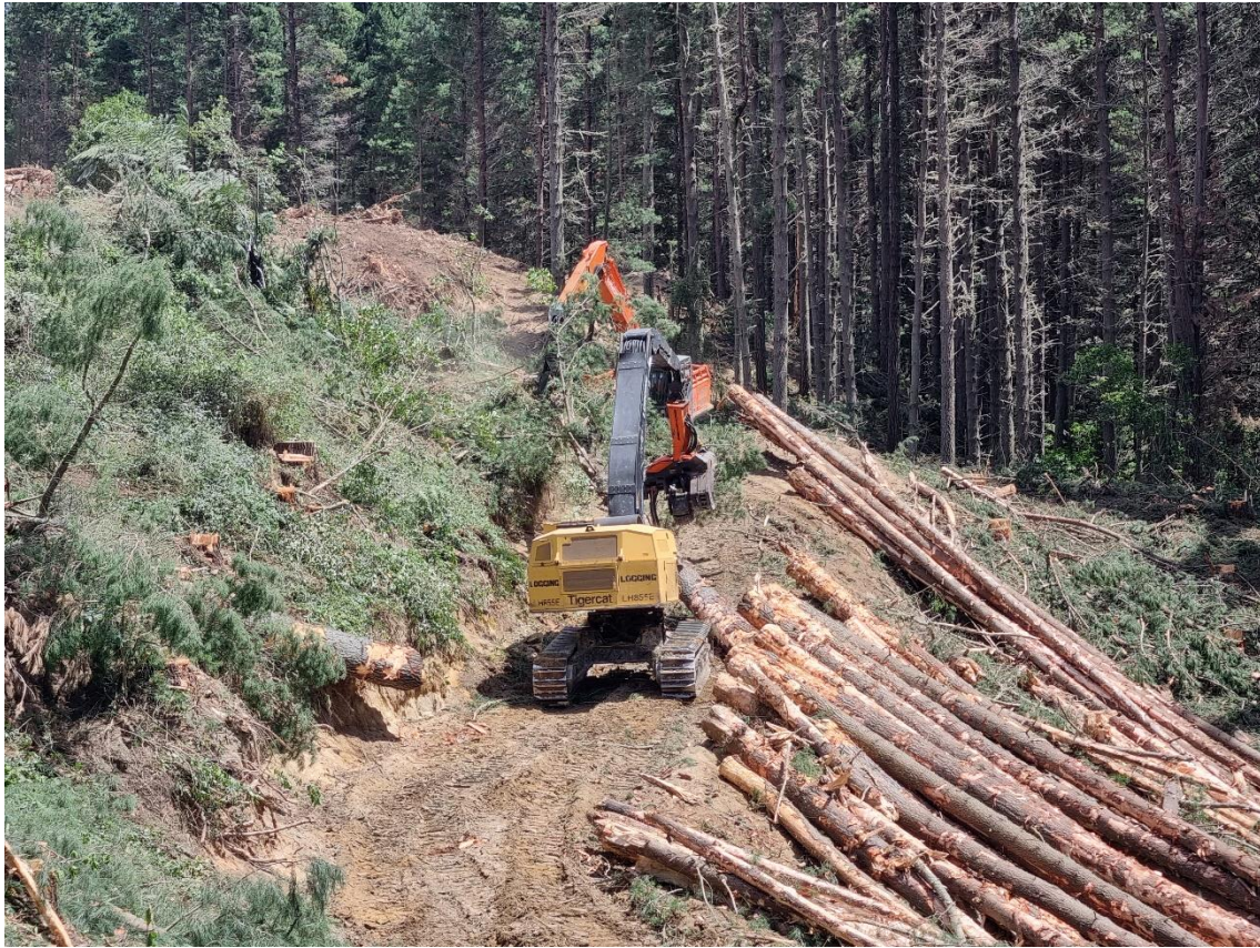
Photo 3: Machines walking out a benched track to help navigate steep terrain and shovel stems to the landing.
