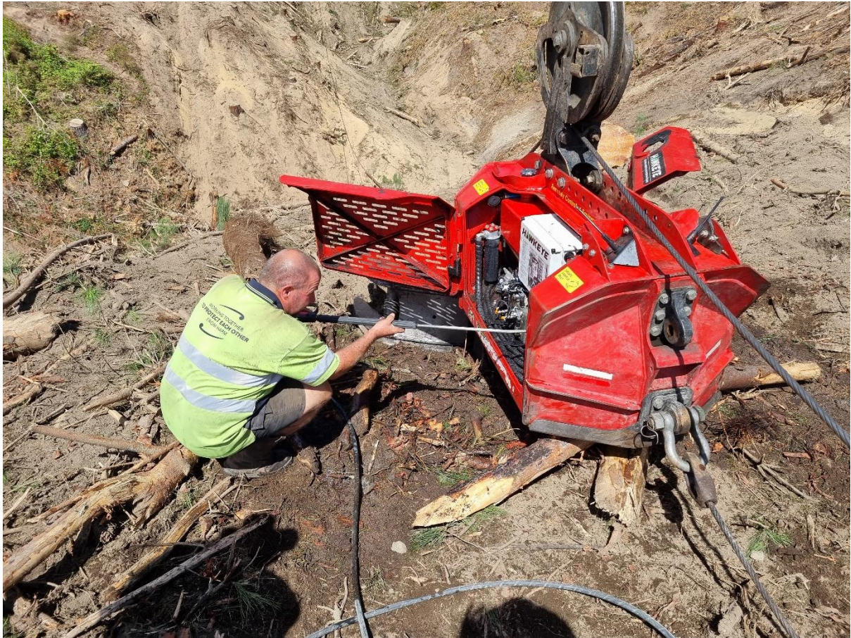
Photo 5: Giving the carriage a good water blasting to remove any built up debris in the fire season.
