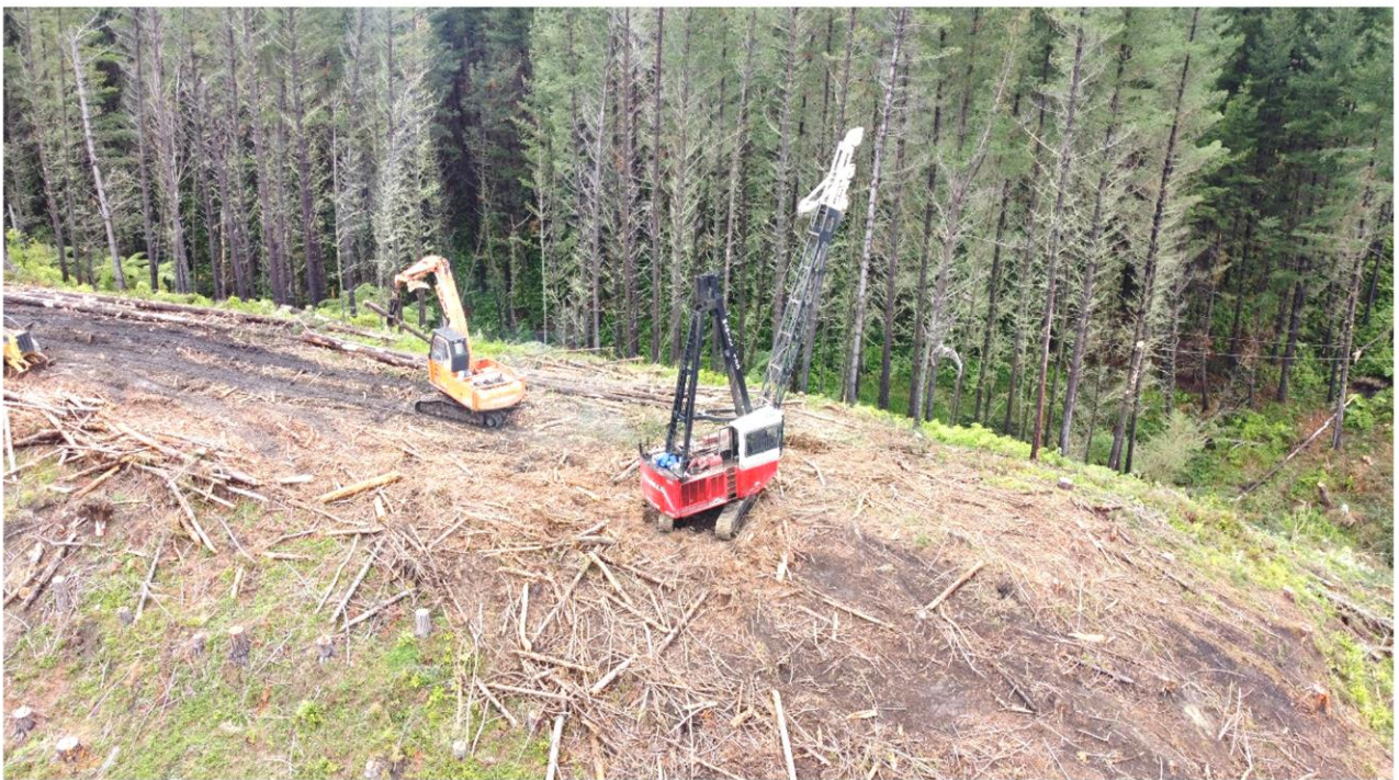
Swing yarder sending grapple out to collect stems.
