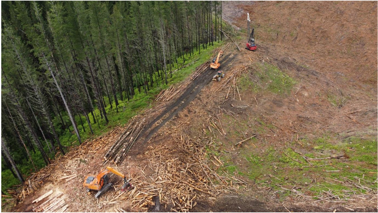
Photo 1: Two-stage operation area between swing yarder and processor.
