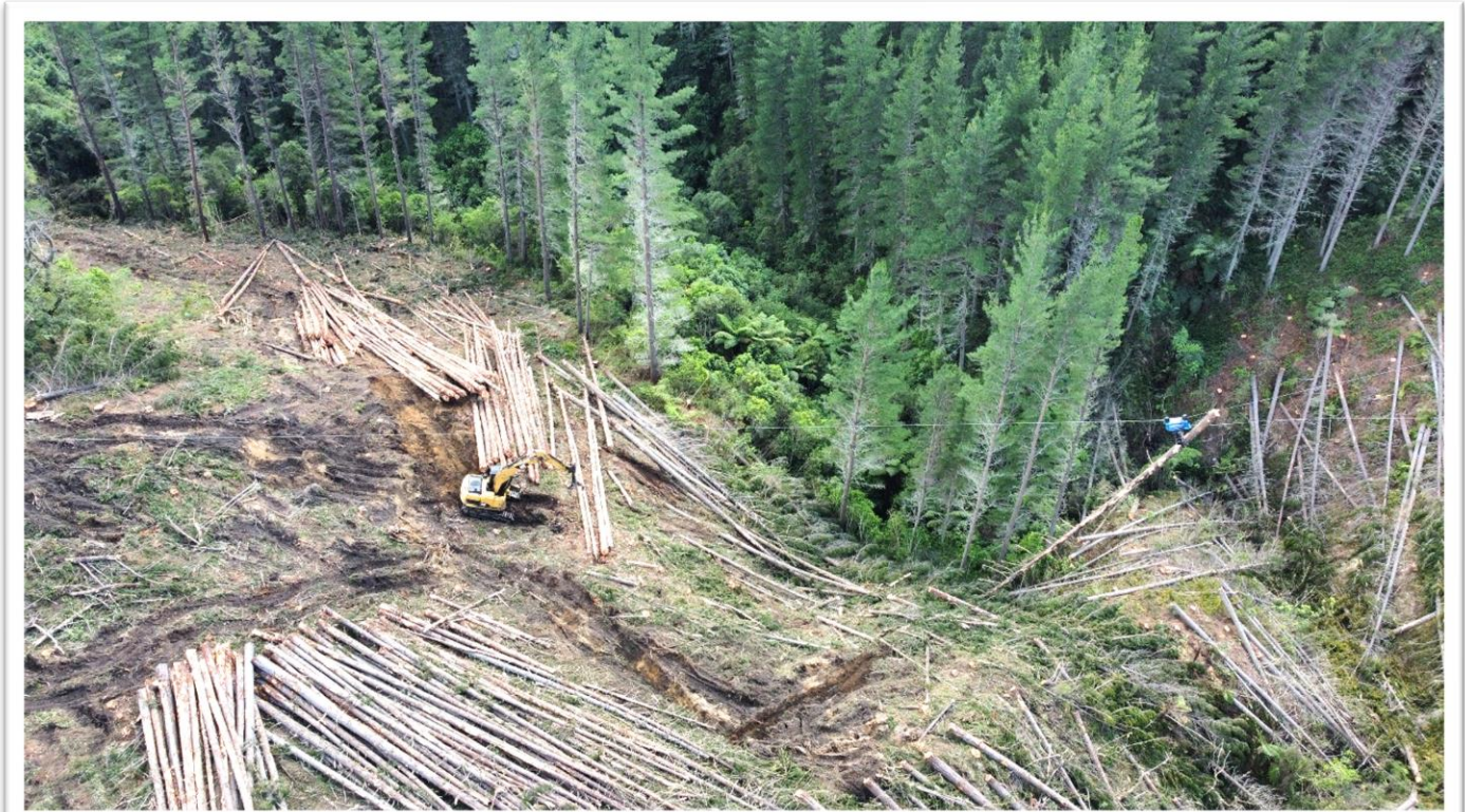
Shovelled wood being extracted in the claws of the grapple.
