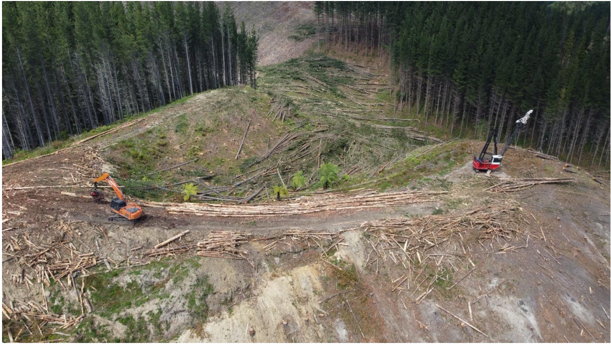
Photo 3: Two-staging stems up to the processing pad.
