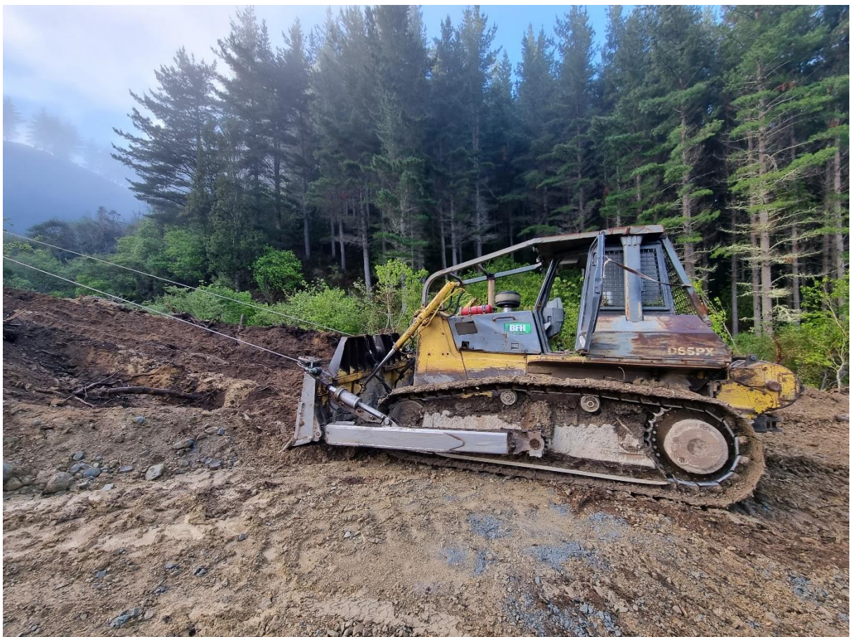
Photo 2: Bulldozer being used as a tail hold for the harvest line.
