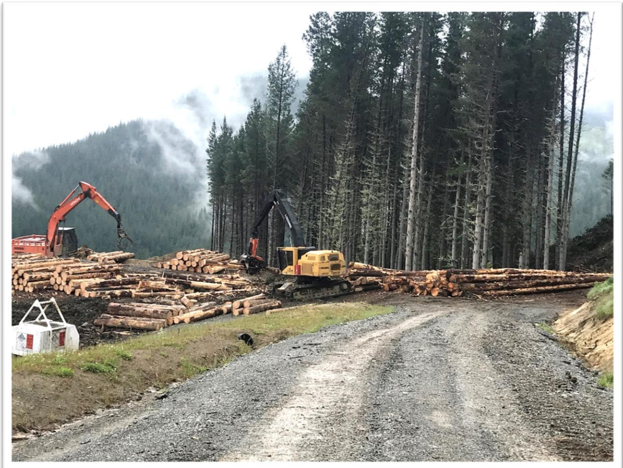
Log 58 processor and loader working on Landing 97.
